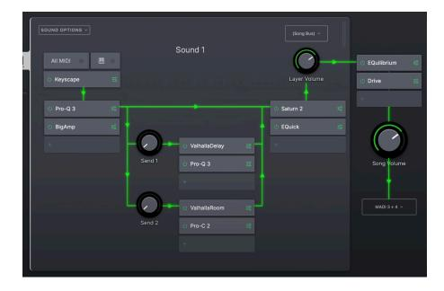
The audio from the instrument flows to the first set of Inserts. 3 FX are allowed in this section.
